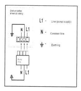
In case of using a water condensates pump it must be connected to the socket located underneath the water pan of the dehumidifier, and only then it is possible to switch it on again.
