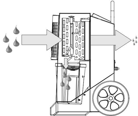
Due to the repeated air circulation through the dehumidifiers, the air humidity is continuously reduced whereby achieving rapid, but gentle drying.
